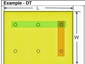
When spacing lights in a structure, a common mistake is to divide the length by the number of lights you want to place, rather than the number of spaces needed.
