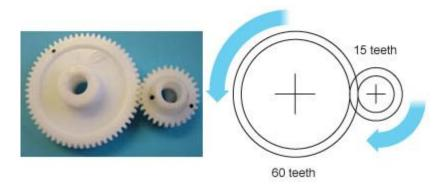
$$Gear\ ratio = \frac{number\ of\ teeth\ on\ driven\ gear}{number\ of\ teeth\ on\ driver\ gear} = \frac{60}{15} = 4$$
