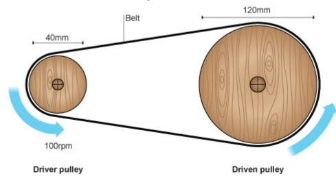
If the pulley wheels are different sizes, the smaller one will spin faster than the larger one. The difference in speed is called the velocity ratio. This is calculated using the formula:
