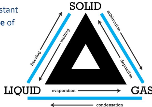
The internal energy is the total kinetic energy and potential energy of all the particles that make up a system. Phase (state) changes occur when particles are moving apart (or closer together) but not moving faster (or slower). This means that the potential energy goes up (or down) so the internal energy goes up (or down) but the temperature stays the same.
