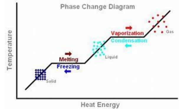
The flat parts of the graph show where the state (or phase) is changing. The energy needed to change the state of 1kg is called the specific latent heat,  $L$ ;  $\Delta E = mL$ . To change from 1kg of liquid to 1kg of gas, the specific latent heat of vaporisation is needed. To change from 1kg of solid to 1kg of liquid, the latent heat of fusion is needed. The temperature does not change when the state changes (hence the flat part).
