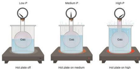
If the temperature of the gas in a fixed volume increases, the pressure increases. The number of molecules stays the same!
