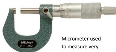
Micrometer used to measure very small widths (0.01 mm)
