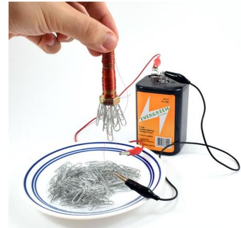
A simple electromagnet can be made by coiling a copper wire (solenoid) round an iron core (like a nail or bolt shown above). This induces magnetism in the core. The strength of the magnetic field can be increased by: i) increasing the current in the wire; ii) increasing the number of turns on the coil\*; iii) Adding the iron core in the first place.
